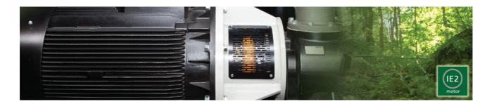
Aydın Trafo coupled series compressors eliminate the disadvantages of compressors operating with belt/pulley system. Minimum transmission loss contrary to the conventional type connections, electric motor and screw block is connected to each other directly in coupled series connections. In coupled compressor interconnected with direct (1:1) drive, transmission loss arising from the power transmission is reduced to zero.
